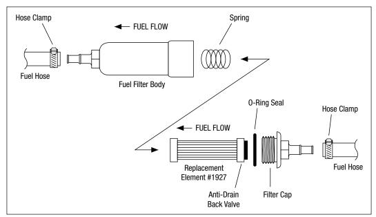
Figure 1 - Fuel Filter Assembly Diagram
